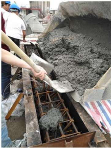
Construction of HSC Column Specimen
