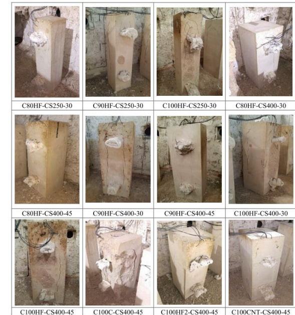
Photos of HSC Samples after Fire Test
