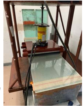
Bending stress test for glass
