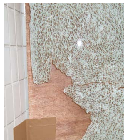
Tempered glass with spontaneous breakage
