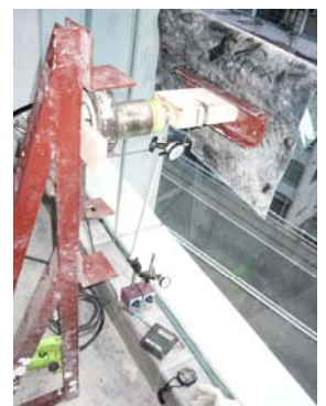
Load test on glass balustrades
